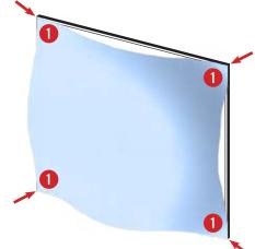
2 CRITICAL: Start from each corner and work towards the center of the frame to evenly distribute the gasket in the frame channel.
