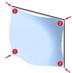
**CRITICAL:** Start from each corner and work towards the center of the frame to evenly distribute the gasket in the frame channel.
