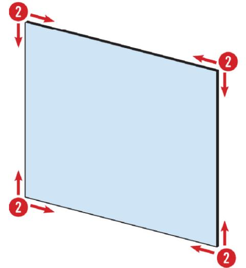
**DO NOT** start at one corner and work in one direction across the frame as this will stretch the gasket and bunch the fabric.
