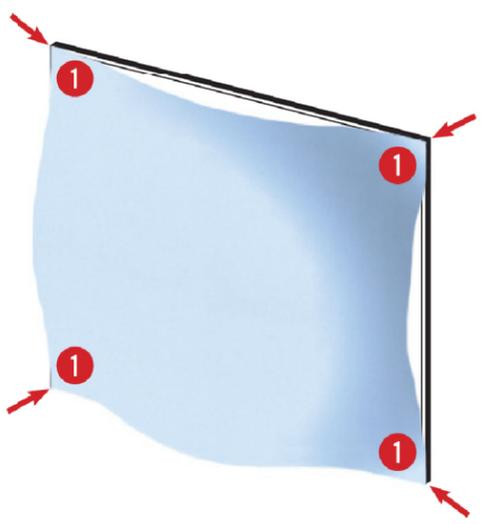
2 **CRITICAL:** Start from each corner and work towards the center of the frame to evenly distribute the gasket in the frame channel.
