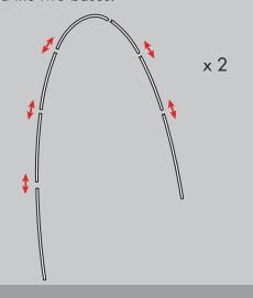
Lay one of the arches on its side. Attach 2. the two base supports.
